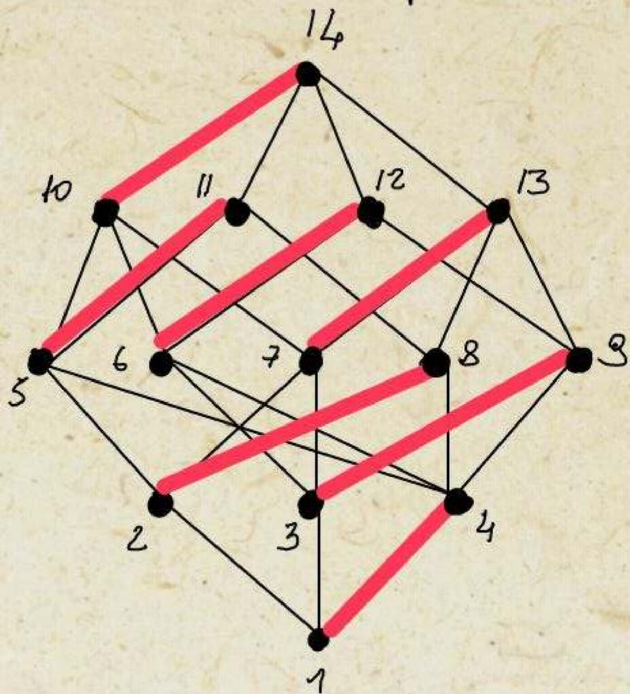
$$R_{1,14} = (q-1)R_{1,10} + R_{4,10}$$
