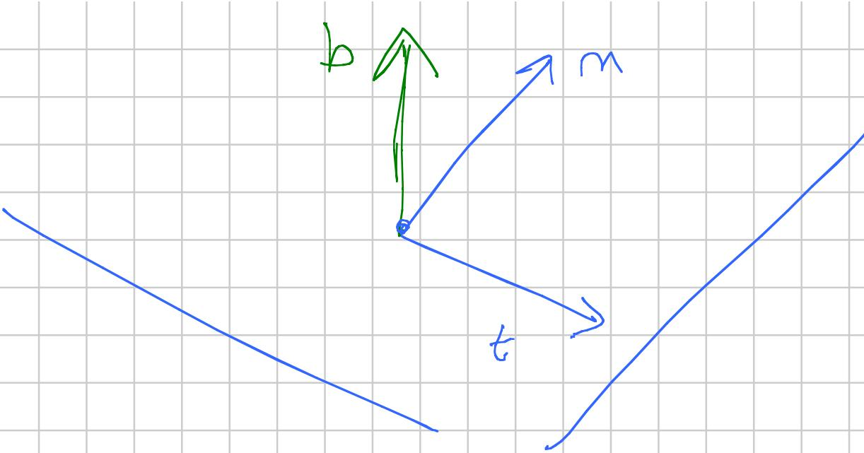
piano osculatore =  $\text{Span}(t, n) = b^\perp$
